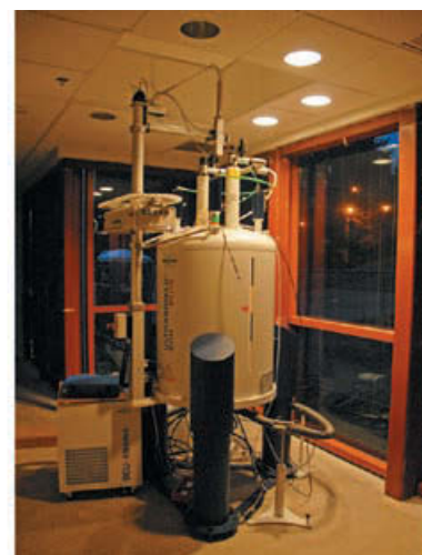
The superconducting magnet of an FTNMR spectrometer.
