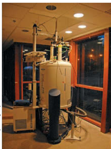
The superconducting magnet of a 500 Mhz FT-NMR spectrometer.
